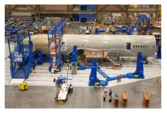
Shadow factories exist for both the 787 and the 737 lines, tackling faults found in finished aircraft. These have included shimming issues, fuselage problems, improperly drilled holes and more. While the 737 MAX line could be some time before reworks are completed, there's a light at the end of the tunnel for the Dreamliner.
